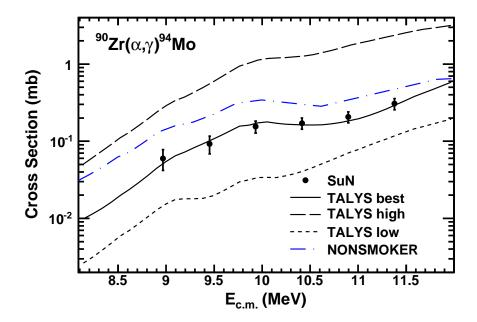
Figure 10.5: Experimental cross sections for the  $^{90}\mathrm{Zr}(\alpha,\gamma)^{94}\mathrm{Mo}$  reaction compared to TALYS 1.6 and NON-SMOKER calculations. The three TALYS curves correspond to the upper limit, lower limit, and best-fit calculations (see text for details).
