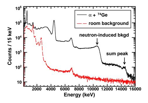
Figure 10.4: Total  $\gamma$ -summed spectrum for an  $\alpha$  beam impinging onto the enriched <sup>74</sup>Ge target at  $E_{c.m.}=8.5$  MeV, with the <sup>74</sup>Ge $(\alpha,\gamma)^{78}$ Se sum peak at 14.5 MeV. The neutron-induced peak around 10.5 MeV comes from neutrons emitted in the <sup>74</sup>Ge $(\alpha,n)^{77}$ Se reaction. Also plotted is the normalized room background spectrum.
