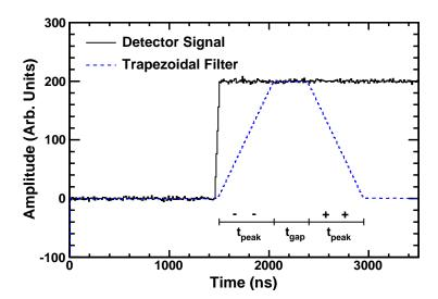
Figure 5.4: Illustrating the use of a digital trapezoidal filter using a signal step function. For every digitized point, the average value of points in the "-"  $t_{peak}$  region get subtracted from the average value of points in the "+"  $t_{peak}$  region. The two  $t_{peak}$  regions are separated by a time  $t_{gap}$ . For a step function, the response is a trapezoidal shape and the height of the trapezoidal filter contains the energy information of the signal.
