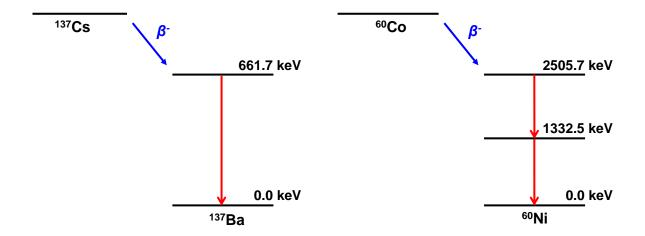
Figure 5.6: Simplified decay scheme showing the dominant decay radiation for the radioactive sources <sup>137</sup>Cs (left) and <sup>60</sup>Co (right).
