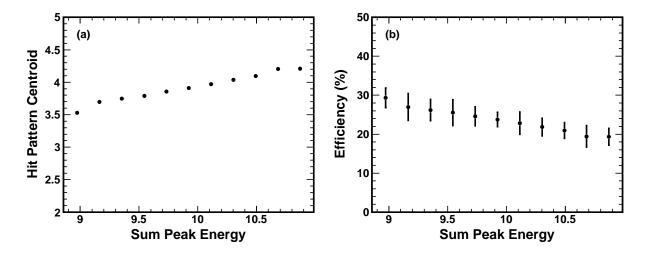
Figure 6.10: Values of (a) hit pattern centroid and (b)  $\gamma$ -summing efficiency plotted against sum-peak energy for the  $^{60}\mathrm{Ni}(\alpha,\gamma)^{64}\mathrm{Zn}$  reaction. For the reactions measured in this thesis, the hit pattern centroid and therefore the average  $\gamma$ -ray multiplicity increase with energy, and the  $\gamma$ -summing efficiency decreases with energy.
