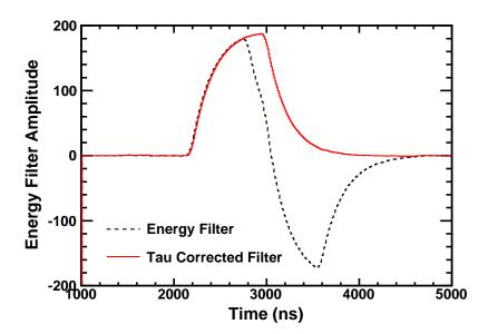
Figure A.2: The response of SuN's tau-corrected energy filter compared to the uncorrected energy filter. By correcting for the exponential decay of the signal, the tau-corrected energy filter does not take on any negative values.
