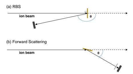
Figure 4.4: General layout of the HIBAL scattering chamber. (a) The RBS detector is located at  $\theta=168.20^{\circ}$ , a distance 4.0" from the target, with a 0.2" diameter collimator in front of it. (b) The rotating detector was placed at a scattering angle of  $\theta=30.0^{\circ}$ , a distance 2.75" from the target, with a 0.2" diameter collimator in front of it. The target was then rotated 75.0° and a 15.0  $\mu$  aluminum foil placed in front of the detector.
