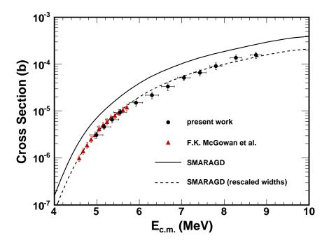
Figure 9.3: Cross section of the  $^{58}$ Ni $(\alpha,\gamma)^{62}$ Zn reaction for the present work (black circles), previous data of Ref. [134] (red triangles), and theoretical calculations from the SMARAGD code [137]. A good description of the data was obtained by modifying the  $\alpha$  width and the  $\gamma$ -to-proton width ratio (dashed line).
