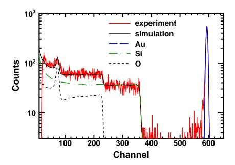
Figure 4.5: Comparison of the SIMNRA fit to an experimental gold-on-glass measurement. The precise beam energy of  $E_{\alpha} = 3804$  keV was determined by fitting the front edge of the gold peak in the spectrum.
