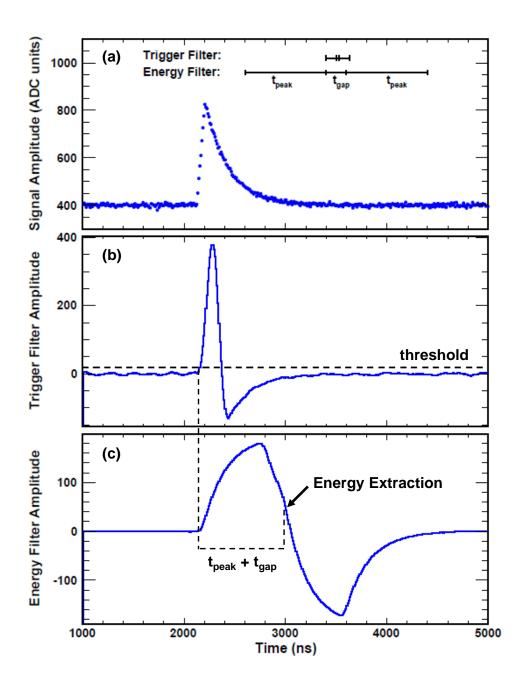
Figure 5.5: (a) Digitized representation of a signal from SuN's PMT after passing through 100 MSPS ADC. (b) Response of SuN's trigger filter. The arrival time of the pulse is obtained when the trigger filter passes above a user-defined threshold. (c) Response of SuN's energy filter. The energy extraction is performed at a time  $t_{peak} + t_{gap} = 800$ ns after the arrival of the pulse, with a correction to the decay constant applied as in Ref. [104].
