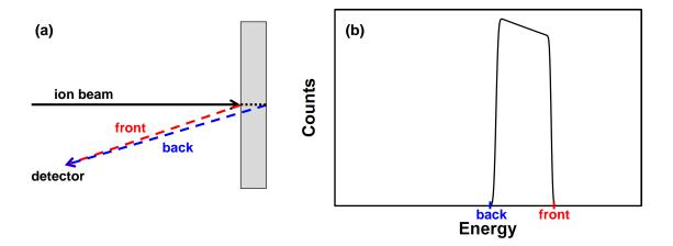
Figure 4.3: Schematic drawing of the RBS technique with (a) an ion beam backscattering off of target nuclei and (b) the energy spectrum of backscattered particles detected by the detector.
