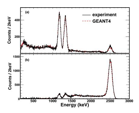
Figure 5.8: Experimental spectrum of SuN taken with a  $^{60}$ Co source with room background subtracted. The result for (a) a segment of SuN and (b) all eight segments are in excellent agreement with GEANT4 simulations. When including the entire volume of SuN, the two sequential  $\gamma$  rays get summed together and the sum peak dominates the spectrum.
