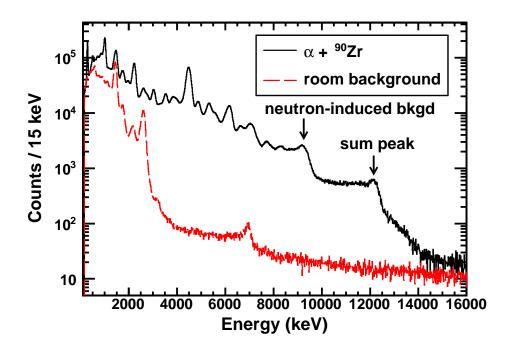
Figure 10.2: Total  $\gamma$ -summed spectrum for an  $\alpha$  beam impinging onto the enriched  $^{90}\mathrm{Zr}$  target at  $\mathrm{E_{c.m.}}=9.94~\mathrm{MeV}$ , with the  $^{90}\mathrm{Zr}(\alpha,\gamma)^{94}\mathrm{Mo}$  sum peak at 12 MeV. The peak around 9 MeV in the spectrum comes from neutrons released in the  $^{90}\mathrm{Zr}(\alpha,n)^{93}\mathrm{Mo}$  reaction. Also plotted is the normalized room background.
