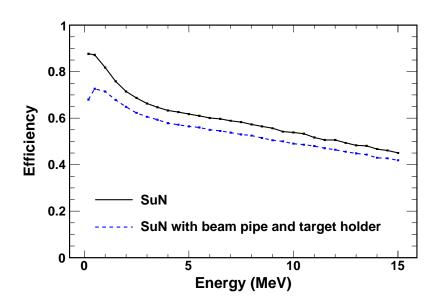
Figure 5.13: SuN's efficiency for the detection of a single  $\gamma$  ray as a function of energy both with and without the beam pipe and target holder used in experiments.
