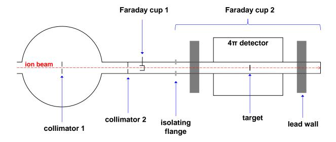
Figure 4.12: Experimental seup for the cross section measurements performed in this dissertation. The dimensions are not to scale.
