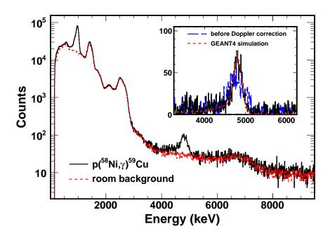
Figure 11.3: Doppler corrected  $\gamma$ -summed spectra for the p( $^{58}$ Ni, $\gamma$ ) $^{59}$ Cu reaction with a comparison to the normalized room background. The inset shows a zoomed in view of the sum peak at  $E_{\Sigma} = 4819$  keV as well as the summed spectrum without Doppler corrections. An excellent agreement with GEANT4 simulation is also observed.
