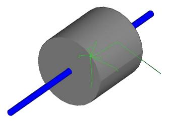
Figure 5.10: Visualization of the GEANT4 SuN detector simulation. The lines inside of SuN are several  $\gamma$ -ray tracks. The one track that scatters outside of SuN does not deposit all of its energy inside of the detector.
