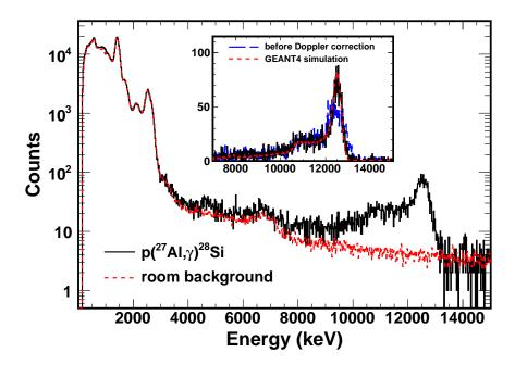
Figure 11.1: Doppler corrected  $\gamma$ -summed spectra for the p( $^{27}$ Al, $\gamma$ ) $^{28}$ Si reaction plotted with the normalized room background. The inset shows a zoomed in view of the sum peak at  $E_{\Sigma} = 12541$  keV. Additionally, the improvement due to applying the Doppler correction is demonstrated and the excellent agreement with GEANT4 simulations is shown.
