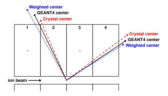
Figure 6.7: Cross-sectional view of the SuN detector showing the different angles used in the Doppler reconstruction. The different angles are to the geometrical center of the NaI crystals, to the weighted center based on the path-length through the crystals, and from SuN's GEANT4 simulation.
