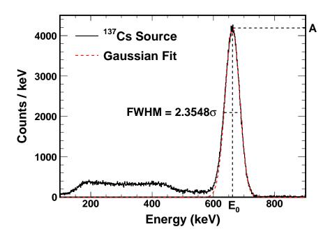
Figure 5.7: Experimental spectrum for a segment of SuN taken with a  $^{137}$ Cs source with room background subtracted. Also shown is the result of a Gaussian fit to the 661.7 keV  $\gamma$ -ray line.
