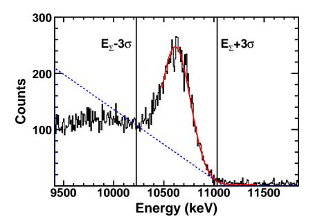
Figure 6.6: Zoomed in view of a typical sum peak from the  $\gamma$ -summing technique with the SuN detector, in this case for the  $^{60}$ Ni $(\alpha,\gamma)^{64}$ Zn reaction. A Gaussian fitting function is used to define a sum-peak region of  $(E_{\Sigma}\text{-}3\sigma,E_{\Sigma}\text{+}3\sigma)$  and then a linear background is determined from an average of the region's boundary values. The sum peak integral is taken to be the number of counts above the linear background.
