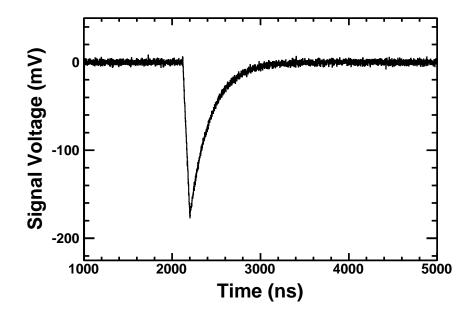
Figure 5.2: Typical signal from one of SuN's PMTs.
