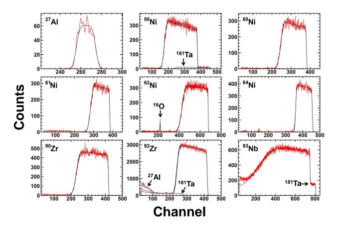
Figure 4.6: SIMNRA fits to RBS spectra of nine of the targets used in this dissertation. The resulting thicknesses are given in Table 4.2.
