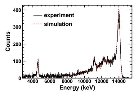
Figure 7.1: Total  $\gamma$ -summed spectrum for the  $E_p = 2517.7$  keV resonance in the  $^{27}$ Al $(p,\gamma)^{28}$ Si reaction. Plotted are the experimental spectrum taken with the SuN detector and the result of GEANT4 simulations.
