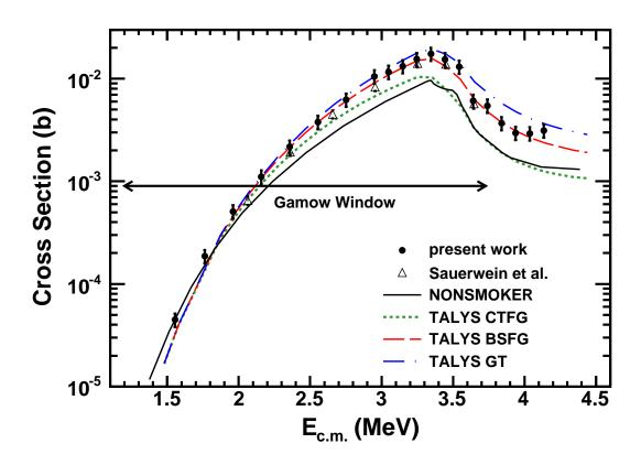
Figure 8.4: Cross section vs. center of mass energy plot for the  $^{74}$ Ge(p, $\gamma$ ) $^{75}$ As reaction. The measurements of this dissertation (solid circles) and previous data of Ref. [74] (open triangles) are compared to theoretical calculations using NON-SMOKER and TALYS 1.4 nuclear reaction codes. The most accurate reproduction of the data is the TALYS backshifted Fermi gas model (BSFG).
