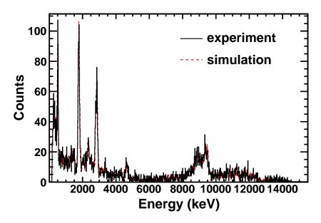
Figure 7.3: Spectrum from one segment of the SuN detector for events in the sum-peak region of the  $E_p = 2517.7$  keV resonance in the  $^{27}\text{Al}(p,\gamma)^{28}\text{Si}$  reaction. Plotted are the experimental spectrum taken with the SuN detector and the result of GEANT4 simulations.
