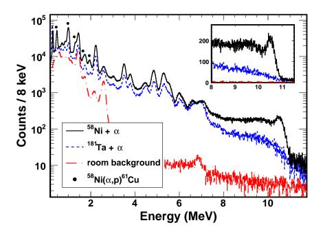
Figure 9.2: Experimental spectra from the SuN detector for measurements at  $E_{\alpha} = 7.7$  MeV. The spectra correspond to <sup>58</sup>Ni (solid black), thick tantalum backing (dotted blue), and normalized room background (dot-dashed red). The inset shows a zoom around the sum-peak region of the <sup>58</sup>Ni( $\alpha,\gamma$ )<sup>62</sup>Zn reaction.
