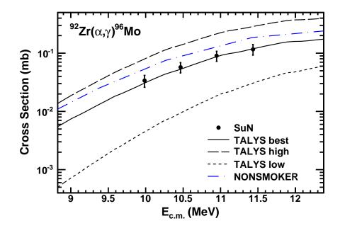
Figure 10.6: Experimental cross sections for the  $^{92}\mathrm{Zr}(\alpha,\gamma)^{96}\mathrm{Mo}$  reaction compared to TALYS 1.6 and NON-SMOKER calculations. The three TALYS curves correspond to the upper limit, lower limit, and best-fit calculations (see text for details).
