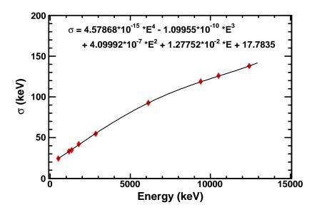
Figure 5.11: Standard deviation in the detected energy of the SuN detector as a function of the  $\gamma$ -ray energy. The points correspond to experimental data and the curve is the best fit function that was implemented in the GEANT4 simulation.
