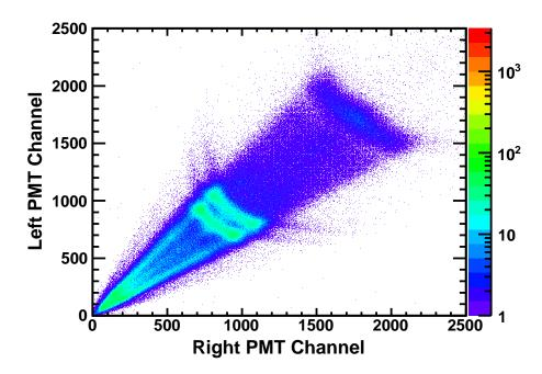
Figure 6.2: Two-dimensional plot showing the response of the left PMT against the response of the right PMT for a  $^{60}$ Co source. The two bands in the spectrum around channel 1000 in each PMT correspond to the two  $\gamma$ -ray transitions in the decay of  $^{60}$ Co. The slope of these bands indicates that the response of the outer two PMTs is affected by where the  $\gamma$  ray deposits energy in the crystal.
