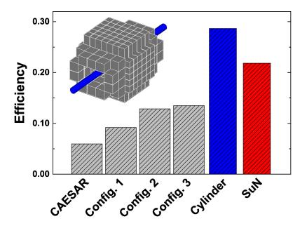
Figure 5.12:  $\gamma$ -summing efficiencies for various configurations of the CAESAR detector (standard configuration inset), a solid cylindrical detector, and the SuN detector for the resonance at a proton energy of  $E_p = 1118 \text{keV}$  in the  $^{27}\text{Al}(p,\gamma)^{28}\text{Si}$  reaction. This resonance deexcites through the emission of 3.2  $\gamma$  rays on average.
