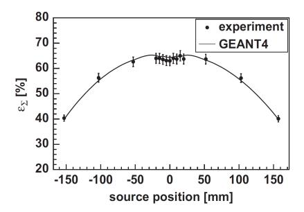
Figure 5.9: Figure from Ref. [77] showing the effect of the location of a  $^{60}$ Co source inside of SuN on the  $\gamma$ -summing efficiency.
