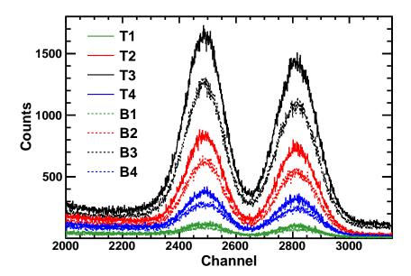
Figure 6.4: The result of gain matching SuN's segments using a <sup>60</sup>Co source. The label T is for the top of the detector and B is for the bottom of the detector. Based on the spectra it can be deduced that the source was place off-center under the third segment of SuN and closer to the top than the bottom.
