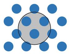
Figure 2.1: Front view of uniformly placed circular targets. The large grey circle represents the area in which projectiles strike the targets.
