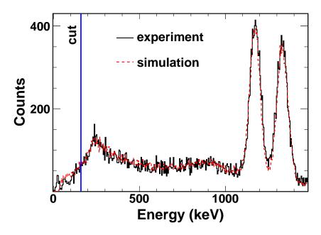
Figure 6.5: Experimental data and GEANT4 simulation for one of SuN's central segments for a  $^{60}$ Co source. In the analysis, a hard cut at 160 keV was applied for each segment in order to use the same threshold in both experiment and simulation.
