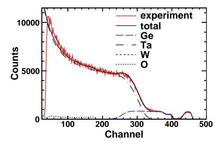
Figure 4.7: SIMNRA fit to the RBS spectrum of enriched  $^{74}$ Ge on a tantalum backing.
