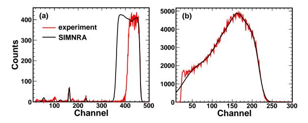
Figure 4.10: Same as Fig. 4.8 with the minimum additional titanium hydride material needed to match the ERD spectrum.
