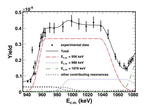
Figure 11.2: Yield curve for the  $p(^{27}Al,\gamma)^{28}Si$  reaction with the experimental data shown in solid circles. The spectrum is dominated by the  $E_{c.m.}=956$  keV resonance, with other large contributions from the  $E_{c.m.}=988$  keV and  $E_{c.m.}=1078$  keV resonances. In this energy region there are additional contributions from the  $E_{c.m.}=856,890,904,966,1051$ , and 1058 keV resonances [110]. The solid line shows the total yield from all resonances.
