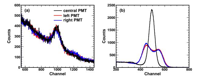
Figure 6.1: (a) Room background and (b)  $^{137}$ Cs source spectra from the three PMT's in a single segment of SuN after gain matching the voltages applied to each PMT. Since the  $^{137}$ Cs source emits  $\gamma$  rays from the center of SuN, the outer two PMTs show a double peak in their spectrum.
