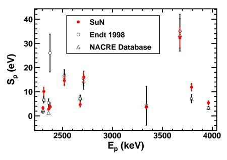
Figure 7.5: Resonance strengths of the  $^{27}\mathrm{Al}(\mathrm{p},\gamma)^{28}\mathrm{Si}$  reaction measured with the SuN detector compared to previous results. Overall good agreement is achieved.
