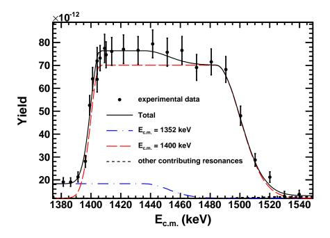
Figure 11.4: Yield curve for the  $p(^{58}Ni,\gamma)^{59}Cu$  reaction. The spectrum is dominated by the  $E_{\rm c.m.}=1400$  keV resonance, with an additional large contribution from the  $E_{\rm c.m.}=1352$  keV resonance. In this energy region there are additional contributions from the  $E_{\rm c.m.}=1496$  and 1514 keV resonances [157]. The solid line shows the total yield from all resonances.
