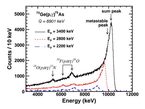
Figure 8.2: Sum peak spectra for three different proton energies  $E_{\rm p}$  normalized to the same number of incoming protons. The location of the sum peak and the metastable peak are indicated for  $E_{\rm p}=3400$  keV.
