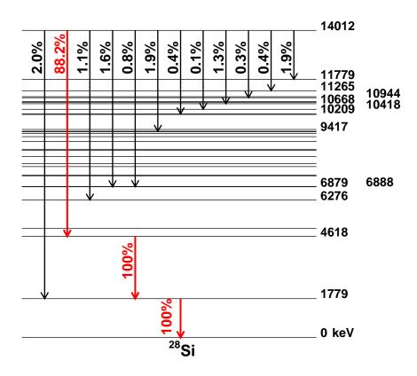
Figure 7.2: Level scheme of  $^{28}$ Si for the  $E_p = 2517.7$  keV resonance in the  $^{27}$ Al $(p,\gamma)^{28}$ Si reaction. For simplicity, only the energy levels and intensities for the primary  $\gamma$ -ray transitions are labeled. The unlabeled levels also participate in the cascades based on their transition probabilities. The most dominant cascade is highlighted and consists of the emission of  $\gamma$  rays with energy 9394, 2839, and 1779 keV.
