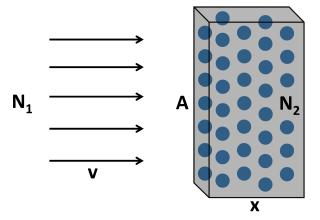
Figure 2.2: A number of particles  $N_1$  and velocity v impinging on a number of particles  $N_2$  within a volume that has area A and depth x.
