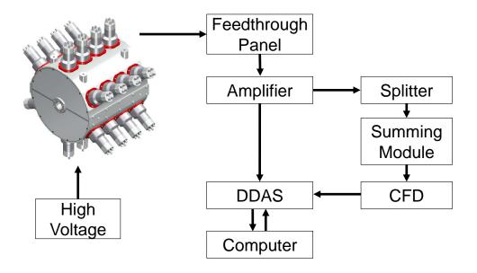
Figure 5.3: Diagram of SuN's data acquistion system.
