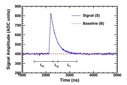
Figure A.1: A digitized signal from the SuN detector plotted along with its baseline. The lengths of the peaking time ( $L_0$  and  $L_1$ ) and gap time ( $L_G$ ) are also drawn.
