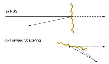
Figure 4.9: Diagram dipicting how wrinkles in the titanium hydride foil may lead to a seemingly larger thickness in the ERD spectra than in the RBS spectra.
