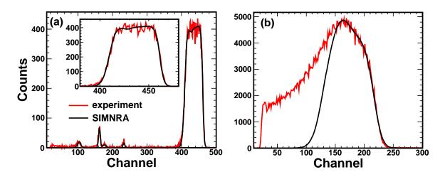
Figure 4.8: SIMNRA calculations compared to experimental data for (a) RBS and (b) ERD spectra of the titanium hydride foil.
