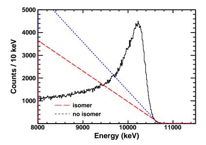
Figure 8.3: Total  $\gamma$ -summed spectrum for the  $^{74}\text{Ge}(p,\gamma)^{75}\text{As}$  measurement at  $E_p=3400$  keV. Also plotted is the linear background with and without including the 304 keV isomer.
